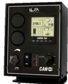
The pumps are controlled by LOFA CP750 panels which provide an auto start/stop function that is triggered by a level transducer. As the level of wet well rises, the pump speed is increased to maintain safe levels during rain events. The control panel is wired to the main VFDs so that the main lift station does not run unnecessarily when the diesel package is running. When the level drops below a set point, the diesel package shuts off.
